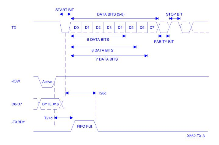
Transmit ready timing in FIFO mode
