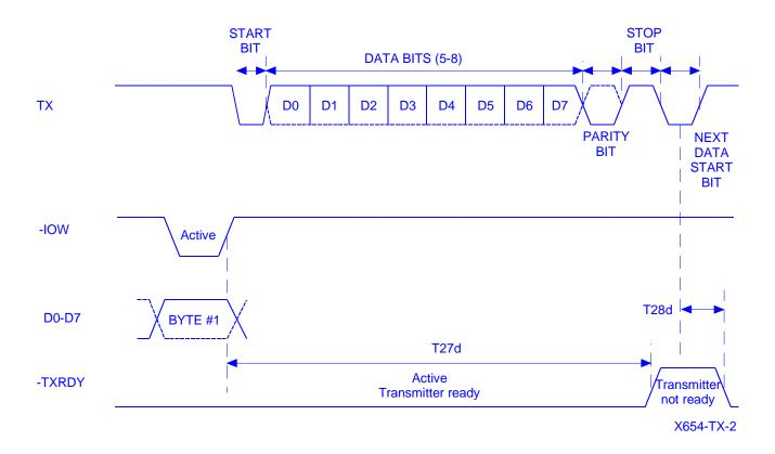
Transmit ready timing in none FIFO mode
