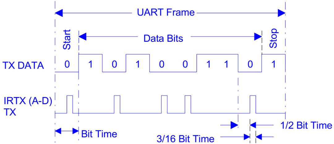
Infrared transmit timing
