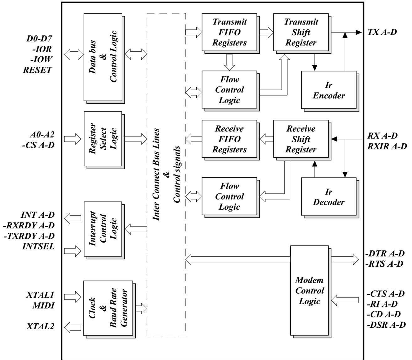
Figure 3, Block Diagram 68 Mode
